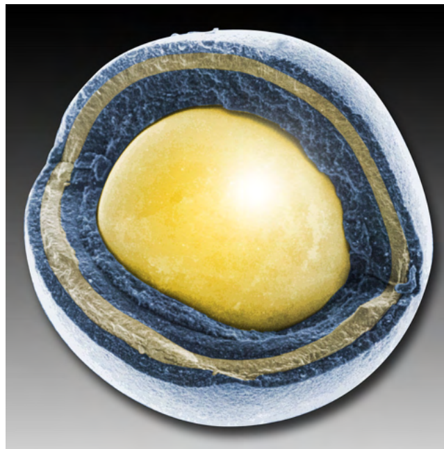
Several advanced reactors will use TRISO fuel, which has a more enriched (20%) uranium-235 core surrounded by a carbide for containment. (Image by INL )
